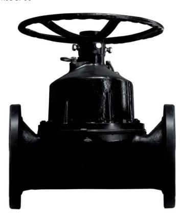
KDV's range of bi directional Straight Through Type diaphragm valves offer exceptional durability and reliability. The clean design completely isolates line media from the mechanical components of the valve. Bubble tight shutoff (Class VI) and in-line serviceability (top entry) maximise plant efficiency and productivity.
