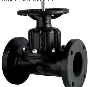
KDV's range of bi directional Straight Through Type diaphragm valves offer exceptional durability and reliability. The clean design completely isolates line media from the mechanical components of the valve. Bubble tight shutoff (Class VI) and in-line serviceability (top entry) maximise plant efficiency and productivity.
