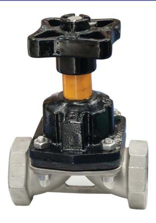
KDV's range of bi directional Weir Type diaphragm valves offer exceptional durability and reliability. The clean design completely isolates line media from the mechanical components of the valve. Bubble tight shutoff (Class VI) and in-line serviceability (top entry) maximise plant efficiency and productivity.
