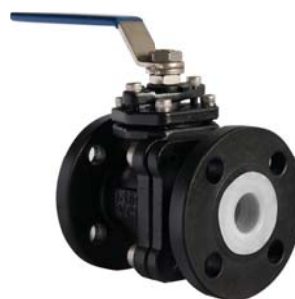
PLASTIC LINED 2 piece - Full Port ANSI 150 (DN15 - DN100) PN10 (DN50 - DN200)
